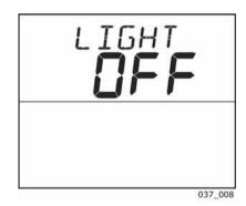
Backlighting is automatically switched off in daylight as part of the instrument's power saving feature and will not operate in daylight.
