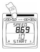
Press and hold for 1 second to enter the timer setup
