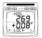
Heading locked at 269<sup>0</sup> now showing +008 change meaning current heading is 277<sup>0</sup>
