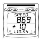
Speed locked at 8.69 kts now showing +10% change meaning current speed is 9.56 kts)
