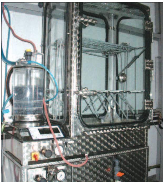
Figure 8.2: Environmental ageing chamber for ammonia atmosphere ageing
